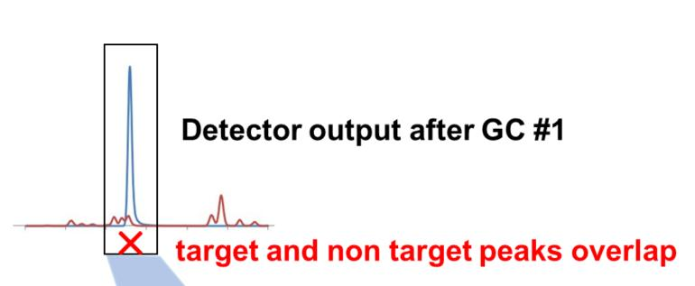
A narrow section of the GC effluent transferred from GC #1 to GC #2
