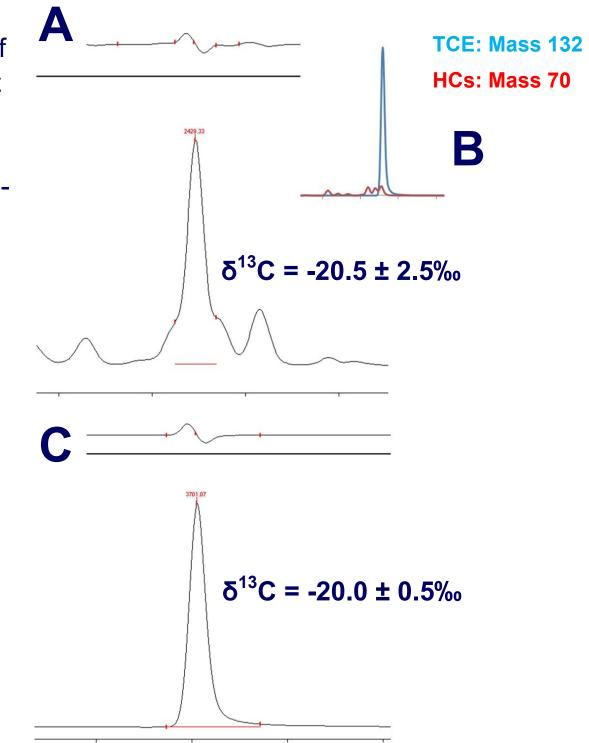
Chromatograms and 45/44 traces of a sample containing Trichloroethene (the target analyte) and a mix of cyclopentane isomers. A) CSIA, standard GC, signal integration uncertainty represents different; B) GCMS, SIM mode; C) CSIA, 2D-GC
