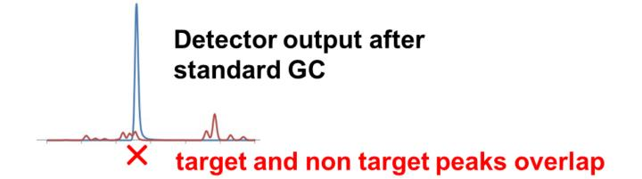
•In standard GC, target compounds are resolved from the non-target compounds using a single GC column. Given the complexity of organic matrix of environmental samples, it is relatively common that more than one compound elute from the GC column at the same time (compound with similar volatility, polarity etc).
