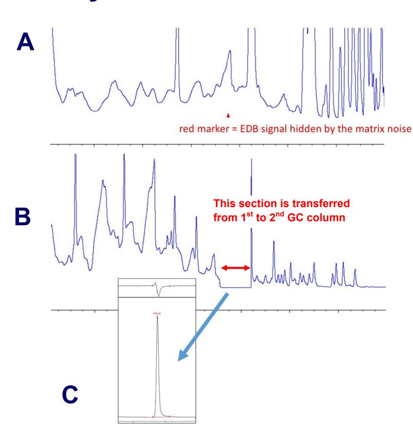
Chromatograms of a sample containing ~ 200 ng of EDB (the target analyte) and several mg of gasoline-range hydrocarbons. A) Standard GC, with EDB marker drawn to represent the amount of EDB-attributable signal hidden by the sample matrix (FID detector, 1st column); B) 2D-GC (FID detector, 1st column) GCMS; C) 2D-GC (IRMS detector, 2nd column).
